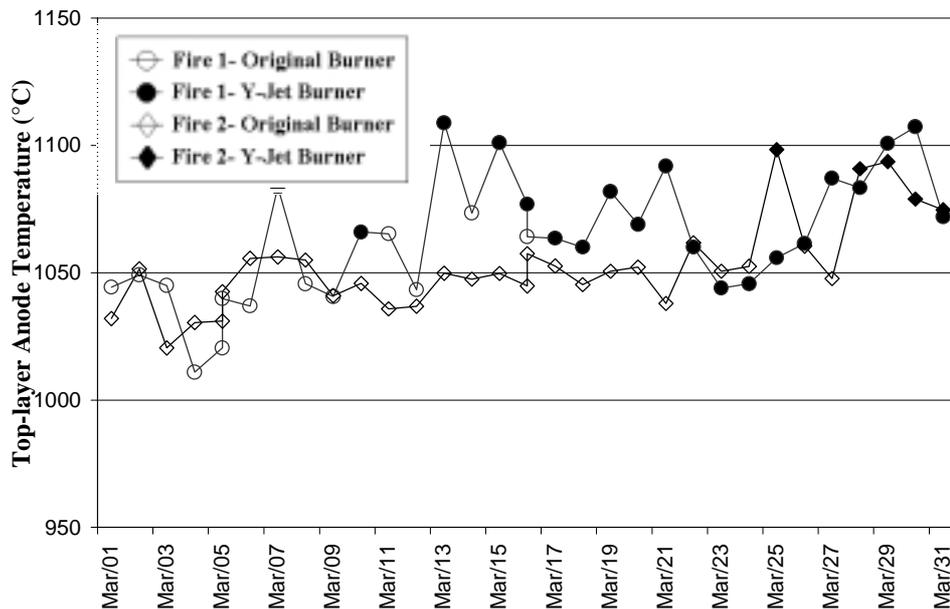
Figure 3- Calcination Temperature of the Anodes from the Top-Layer.
