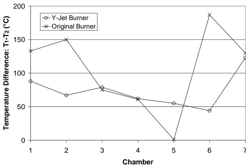
Figure 6- Temperature differences between areas of each chamber.
