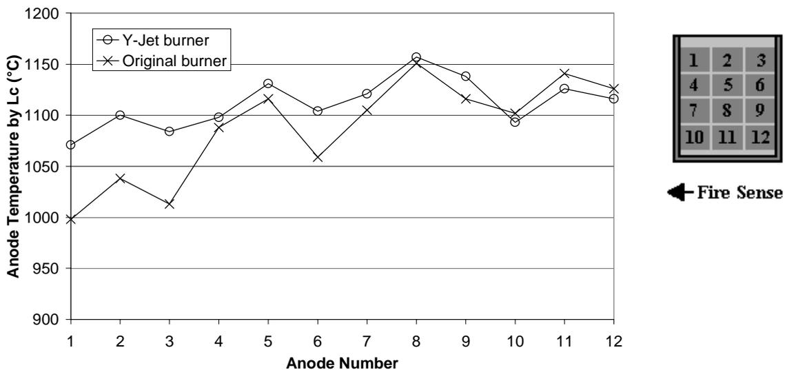
Figure 4- Anode temperature by  $L_c$  method
