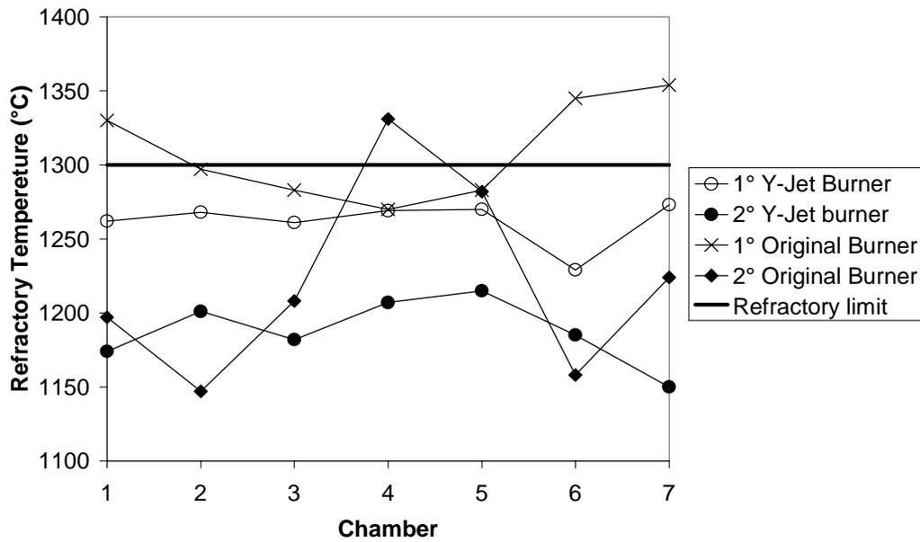
Figure 5- Chamber refractory brick temperature below burners
