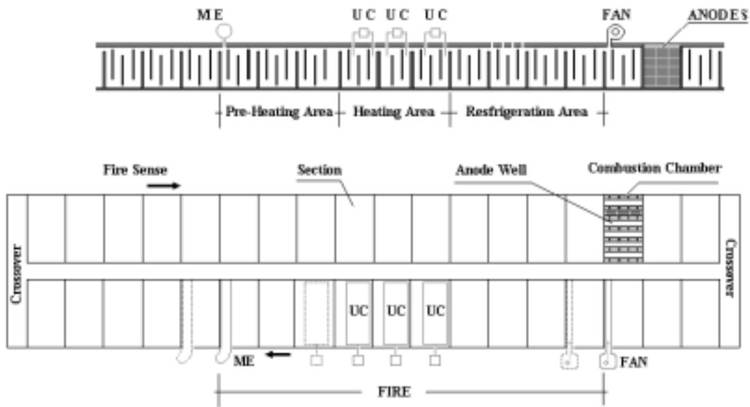
Figure 2- Schematic view of an Albras bake furnace with 36 sections.
